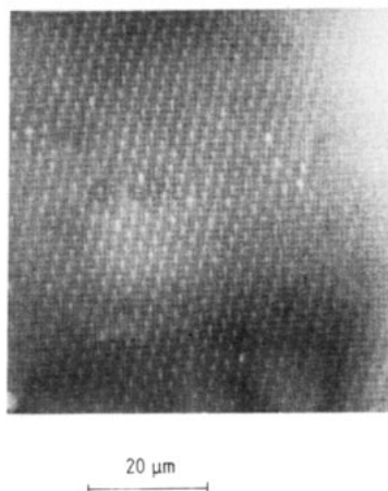
Figure 7. Micrograph of the second layer of the colloidal crystal of 0.53\ \mu\text{m} diameter particles. Integration time is 160 ms. Particle concentration is 0.73 volume per cent. A number of aggregates brighter than the single particle are found in substitutional positions.
